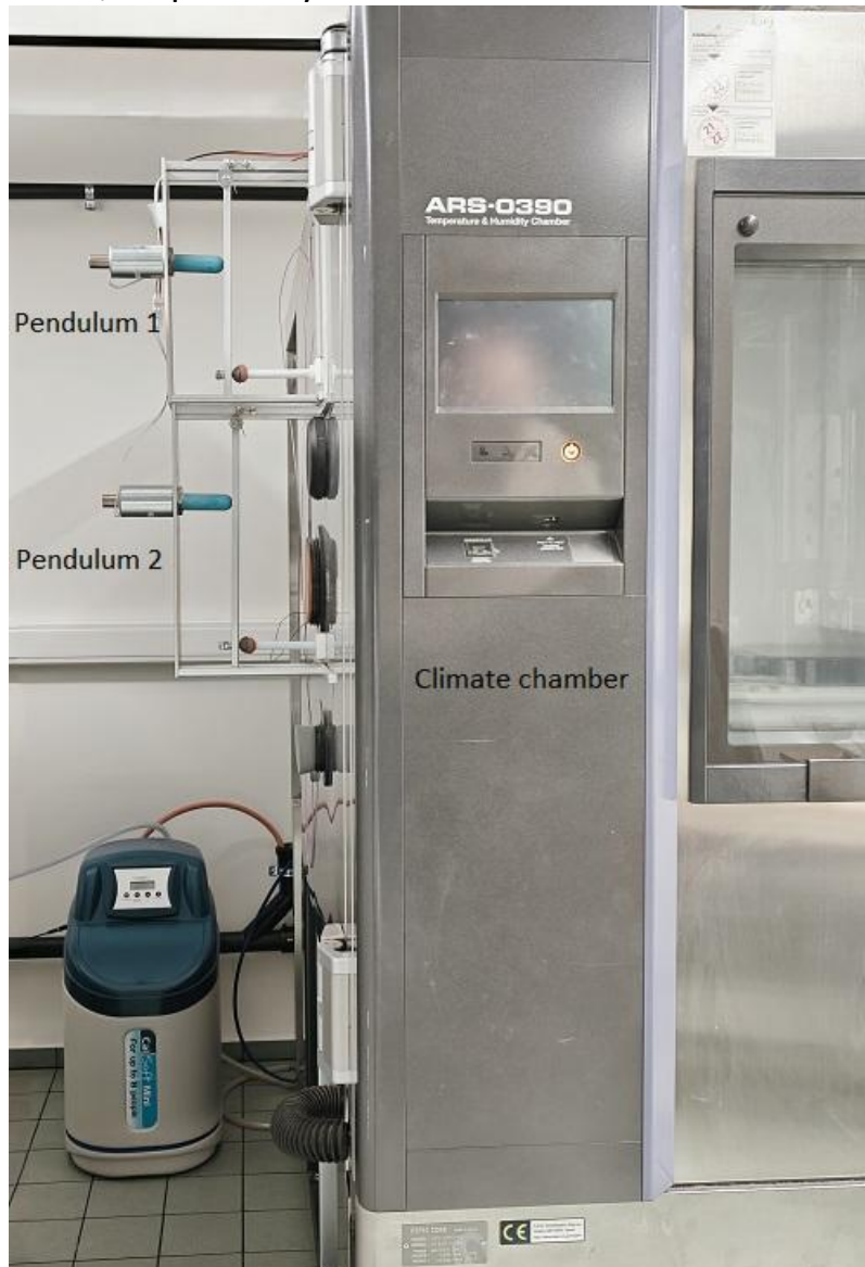
Figure 6.5. Climate chamber with pendulum units on channels 1 and 2
