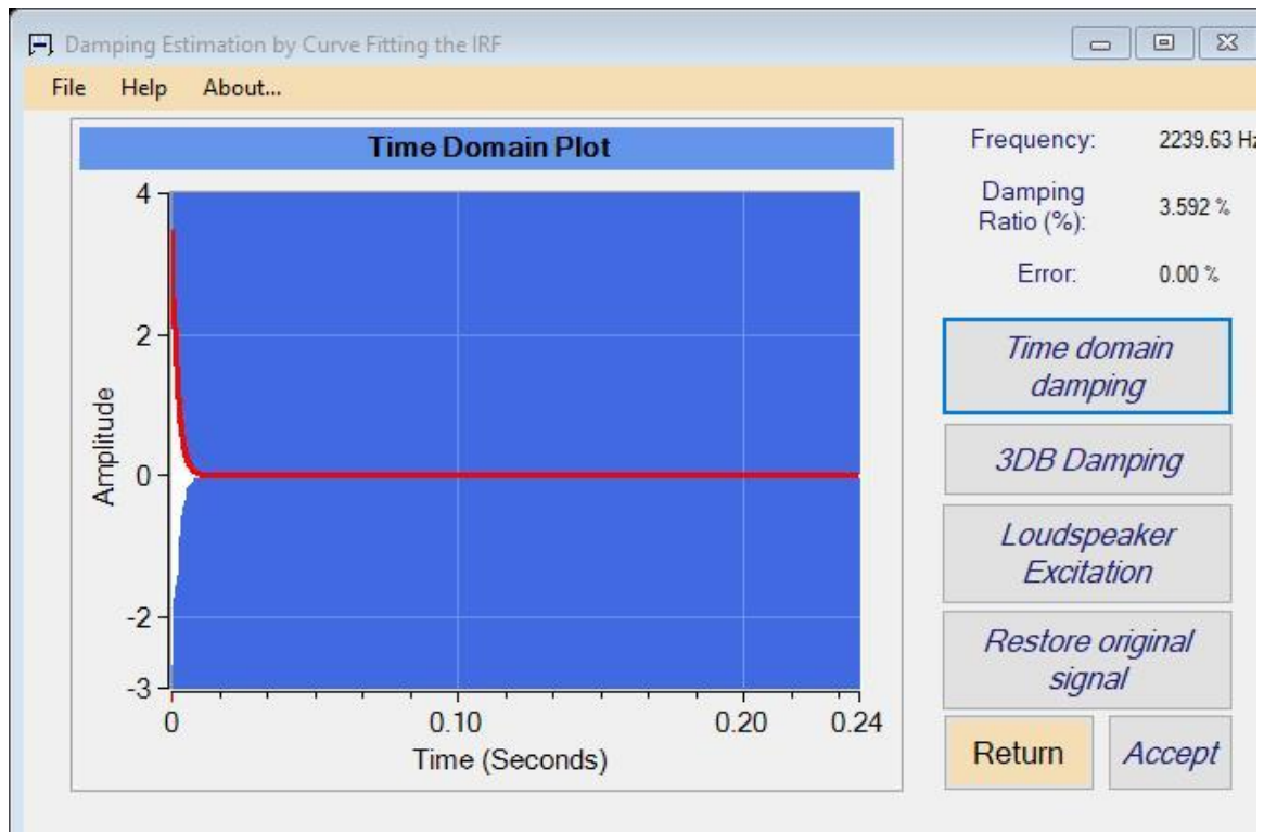
Figure 3.4.1.3. Identification of the damping ratio by curve fitting in the time domain.
