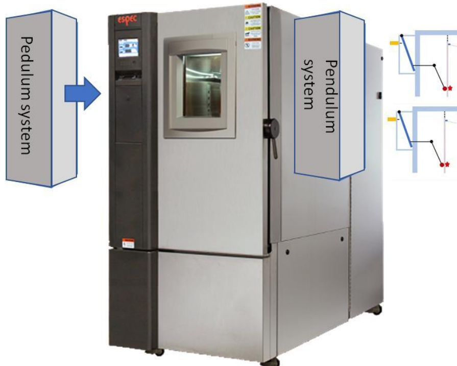
Figure 8.2.1. Climate chamber with pendulum excitation
