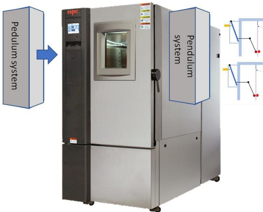
Figure 7.1. Climate chamber with pendulum excitation
